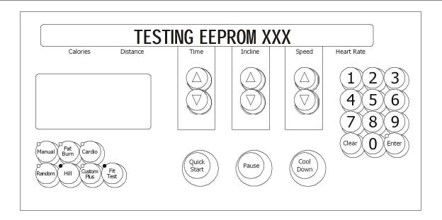
This test allows the user to test the frame tag EEPROM. This test will read/write/replace all used locations in the frame tag EEPROM. If there is an error, the bad location will be displayed. The following is a list of current information that can be seen. If an error has occurred, refer to the troubleshooting section for corrective action.
